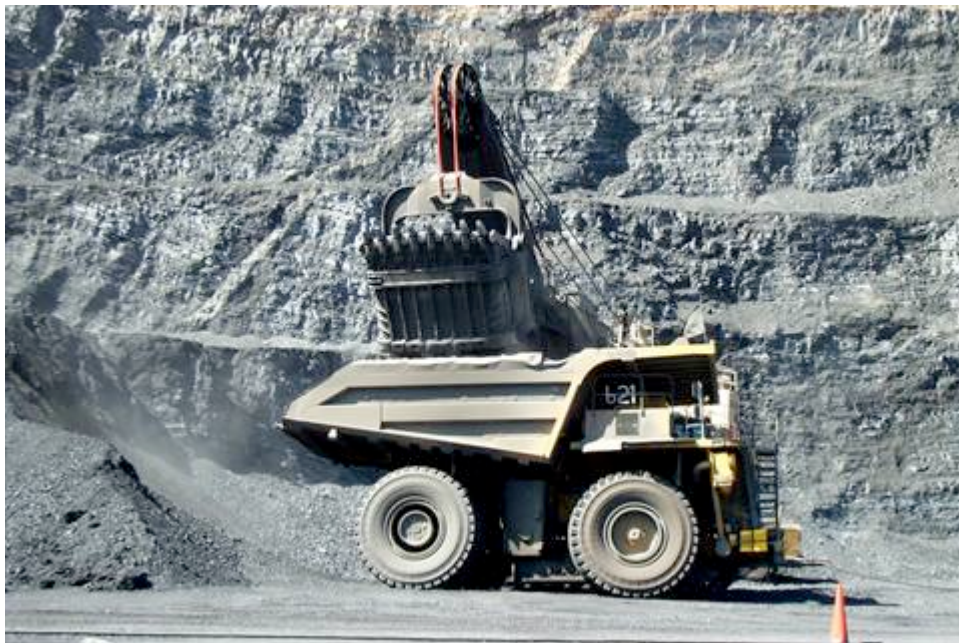
Figure 4. Typical waste loading
