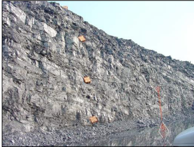
Figure 3.25 - Laser surveying was used to establish true burdens along the face from the crest to the toe.
