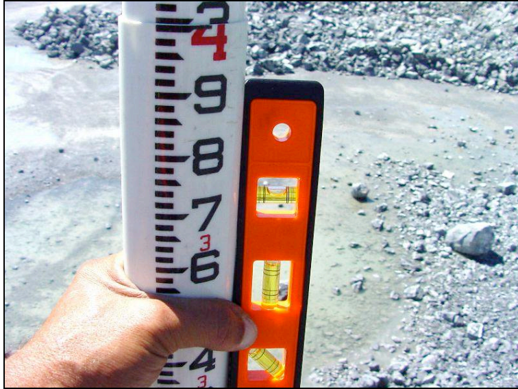
Figure 3.23 - Plumbed survey rod. It was essential to have the survey rod plumbed accurately before a reference line could be shot and transferred down to the toe.
