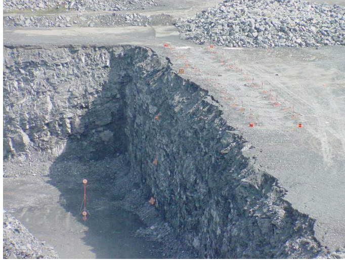
Figure 3.36 - Illustrates a completed shot setup with dimensional and time controls readied for monitoring and analysis
