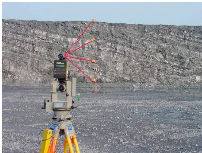
Figure 3.26 - Laser surveying was also used to establish the coordinates of the face markers relative to the vertical hole, bench height and true burdens.
