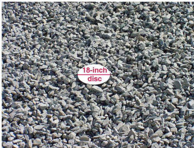
Figure 3.66 - Example of good rock size resolution for the close-up view in relation to the dimensional control size. Here the white circular dimensional control was an 18 inch disk and the known rock size was 4 to 5 inches. Fragmentation analysis on this frame produced a P50 passing size of 4.4 inches with a very narrow (i.e., steep) cumulative percent passing curve.
