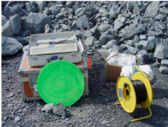
Figure 3.41 - The VODR-1 System ( a TDR based VOD instrument) was used for all measurements. A special foam dielectric coaxial cable was used to measure the PowerPlug speed and gas front velocity in the airdecks. Standard RG-58 coaxial cable was used to measure the VOD of the explosive columns.
