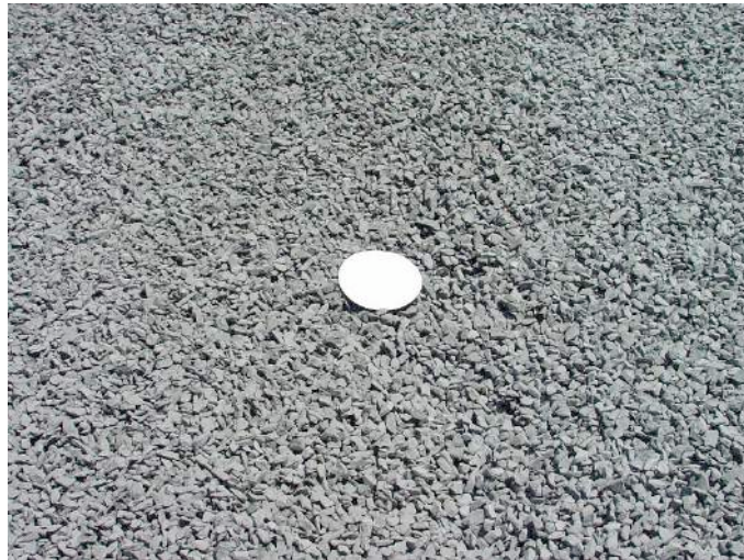
Figure 3.65 - Example of poor rock size resolution for the wide angle field of view in relation to the large dimensional control size.
