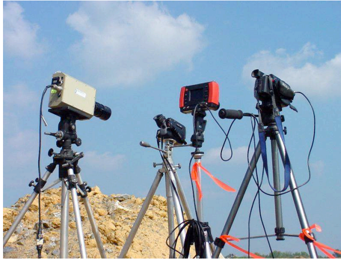
Figure 3.31 - High-speed video camera, high-speed 16 mm film camera and camcorder field setup.
