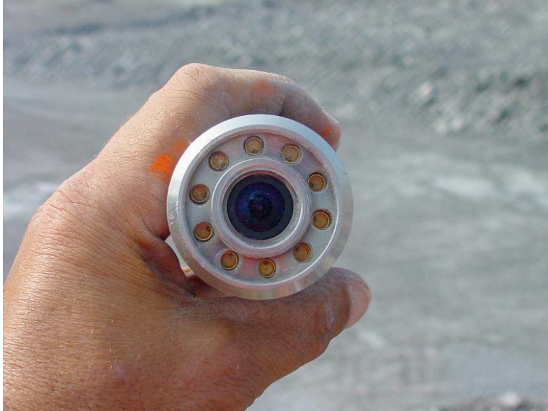
Figure 3.12 - Borehole camera is equipped with integral built-in lights which are adjustable for the lighting intensity required. Different camera heads can accommodate inspections in hole diameters from 2 to 12 inch diameters in B/W or color, and up to 2,000 foot depths.
