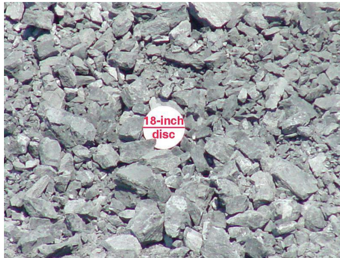
Figure 3.67 - Illustrates the sampling technique which was used to achieve the correct ratios of the image field of view to the dimensional control (disc size) and desired rock size resolution.
