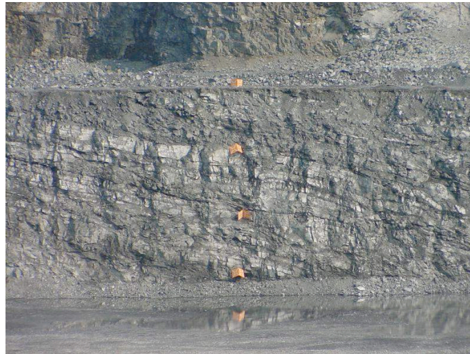
Figure 3.33 - Bench face markers were hung down the face for tracking purposes and to measure the initial velocity, ejection angle, TMIN (rock response time) and cast distance.
