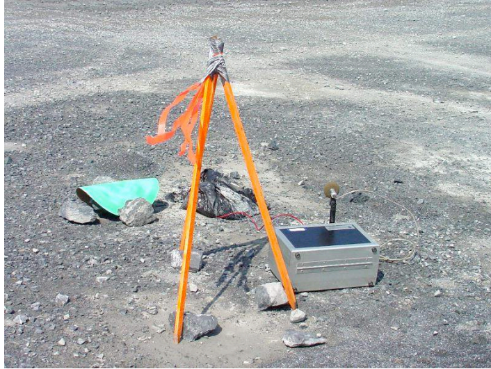
Figure 3.52 - Two types of digital seismographs were used. The close-in geophones to the test shots had a sand bag placed on top of them to assure good coupling with the ground.
