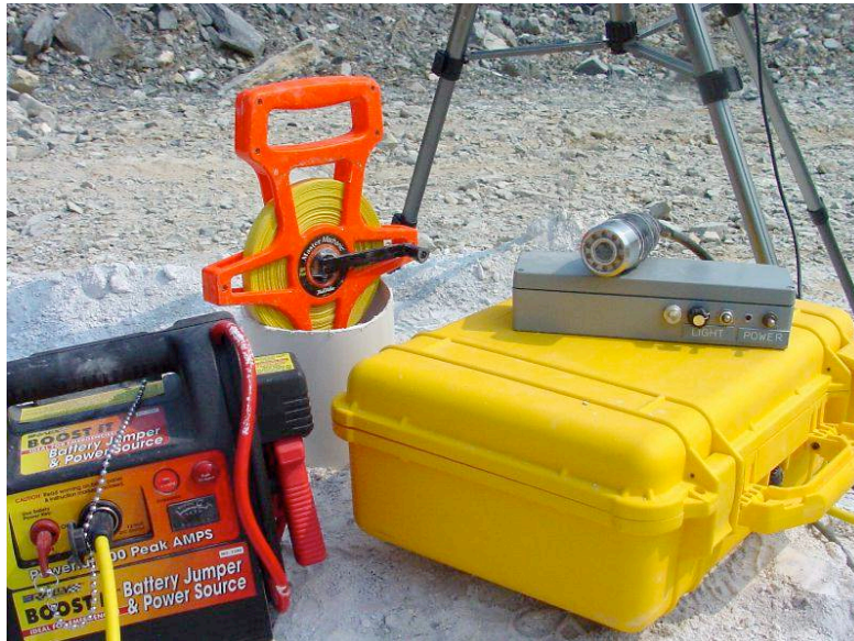
Figure 3.11 - Portable borehole inspection camera system used to probe and document the condition of each monitored test hole.
