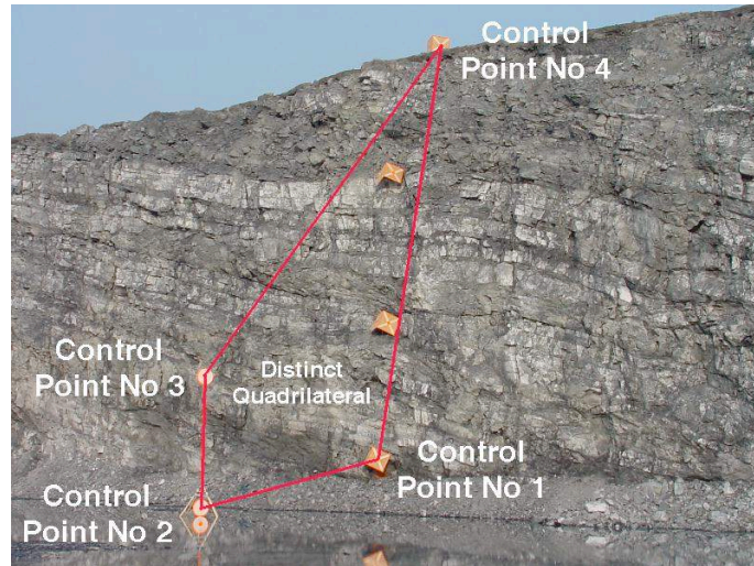
Figure 3.32 - Placement of bench face markers for tracking purposes and how the four control points were established for accurate motion analysis.
