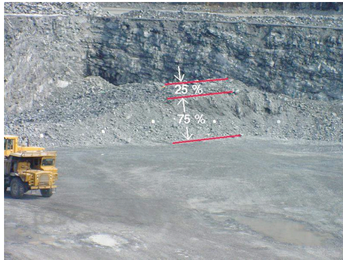
Figure 3.61 - Sampling procedure for each muckpile analysis used 25% of the digital images from on top of the muckpile, and the remaining 75% were taken over 4 cross-sections throughout the muckpile.
