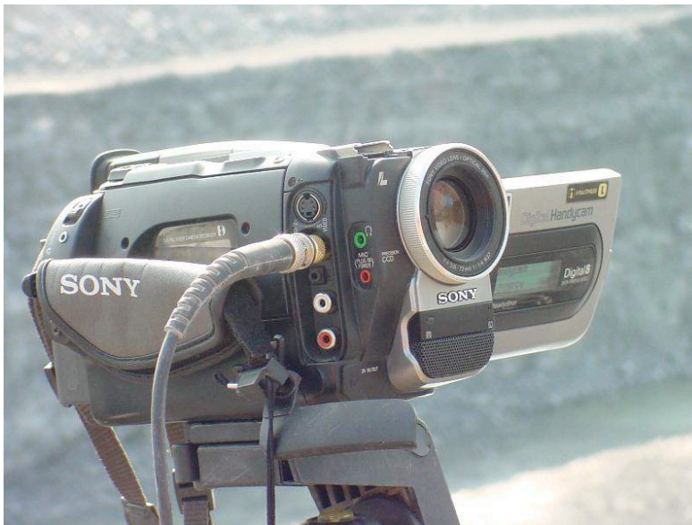
Figure 3.13 - A standard camcorder is used to record the video sequence for each inspected borehole inspection for archiving and later analysis
